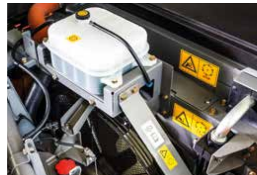
The expansion tank prevents engine parts from overheating.
