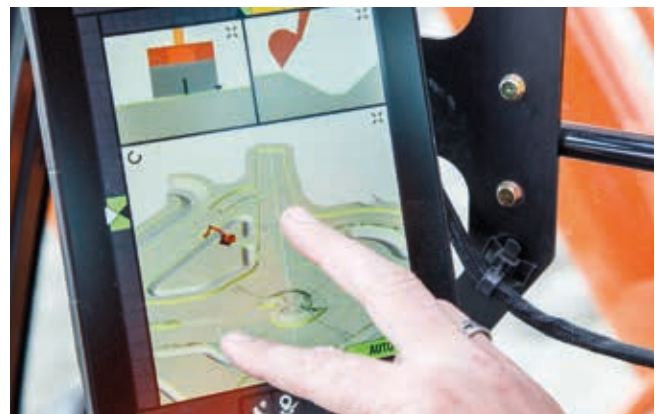
Operators can rotate, or zoom in and out of, the view on the monitor using the touchscreen.
