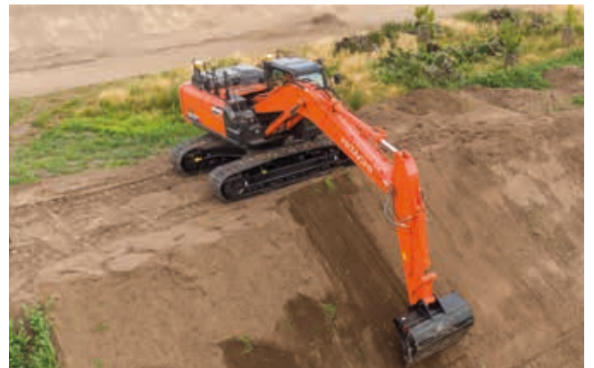
Bucket angle retention mode enables slopes to be completed more quickly.
