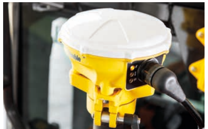
GNSS receivers are used to measure the excavator's position in real time.
