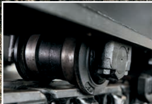
Redesigned lower roller prevents mud entering and causing damage.
