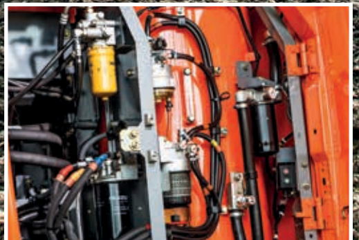
Improved performance derived from the fuel circuit.
