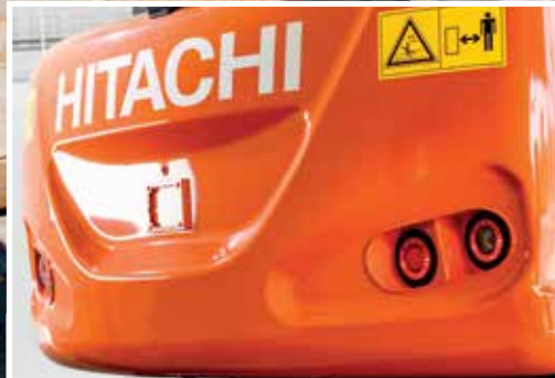
LED tail lights are easily maintained.
