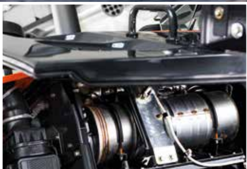
The SCR system reduces emissions.
