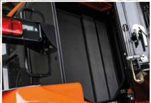
Optional anti-clogging radiators enhance durability.
