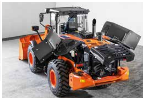
Easy access for maintenance from ground level.
