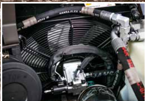
Engine fan helps to reduce emissions and improve fuel efficiency.
