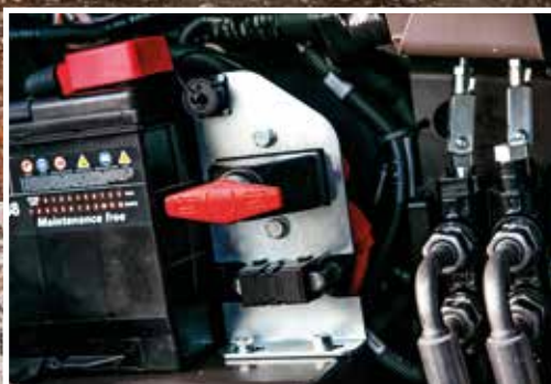
Battery disconnect switch for easy maintenance.
