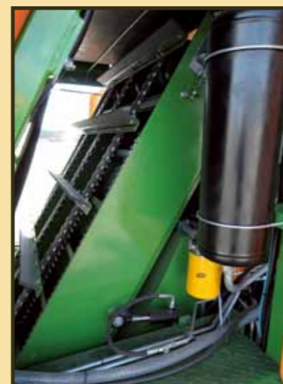
Mechanical waste transport system
