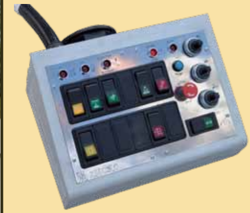
Easy to operate control panel in driver's cab
