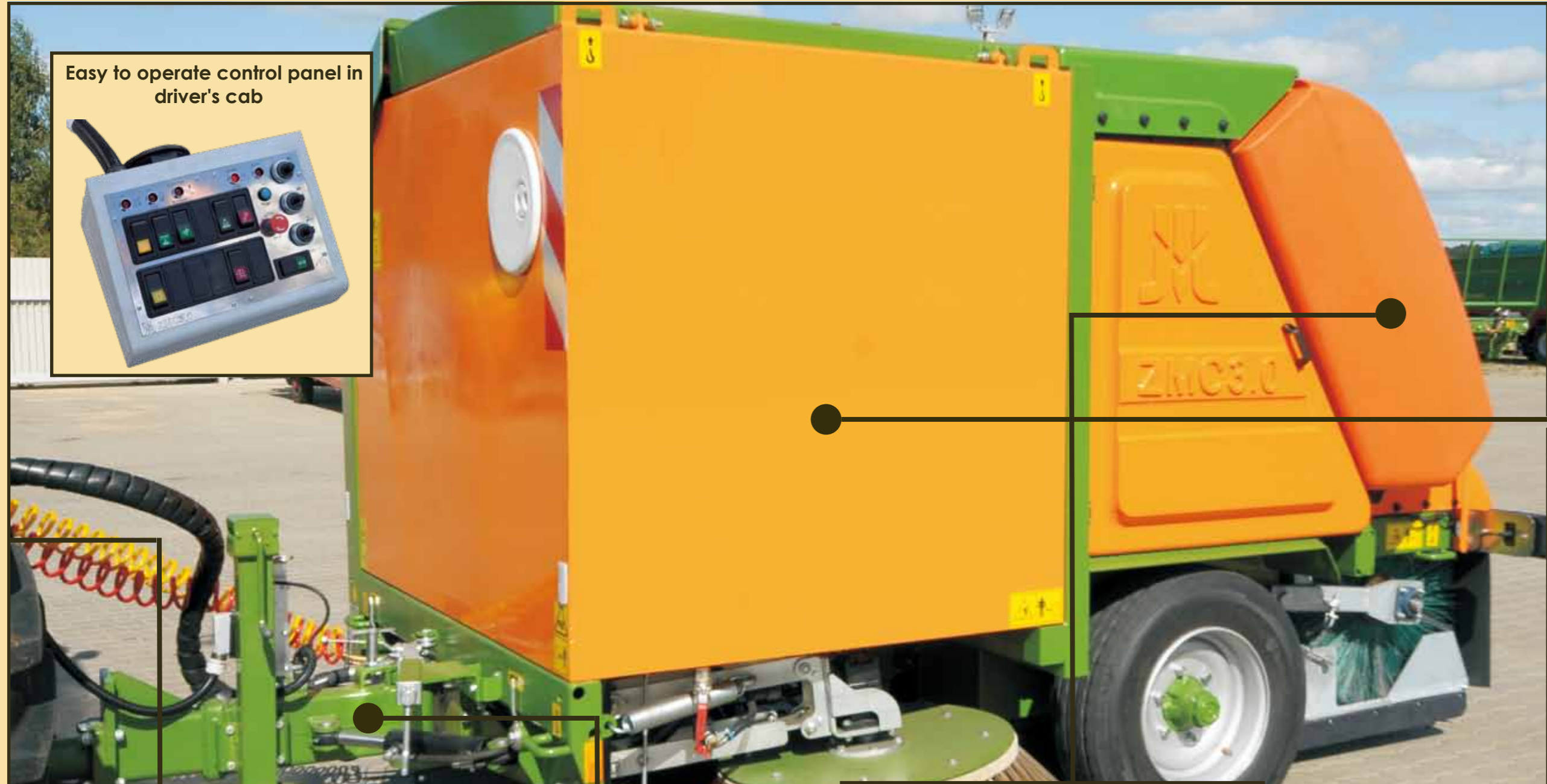
Water tank capacity of 1150dm 3
