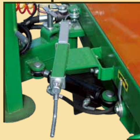
Adjustable drawbar steered via tractor hydraulic system
