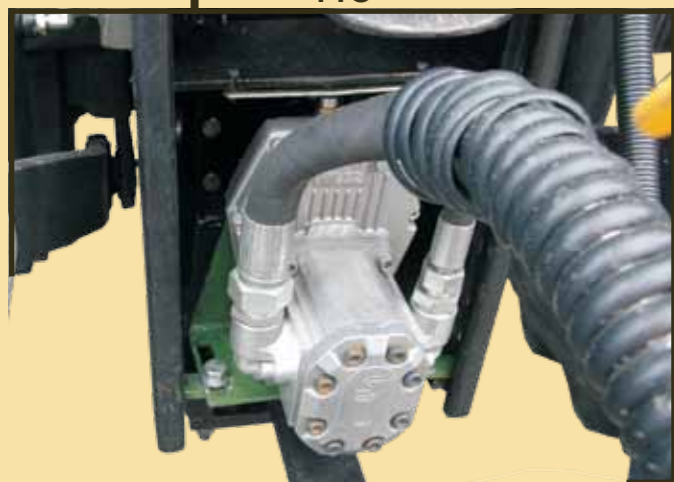
Power supply - hydraulic pump with overdrive (multiplier) attached to rear PTO
