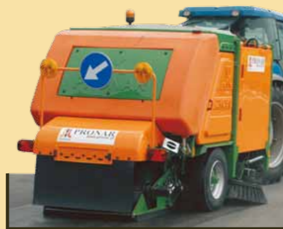
Rear warning lights with additional sign
