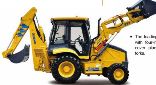
The loading end can be equipped with four-in-one bucket, manhole cover planer, snow shovel, and forks.
