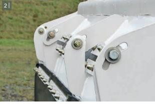
1 The combination of rotor plate with spring assembly and adjustable levelling blade guarantees optimum results.
