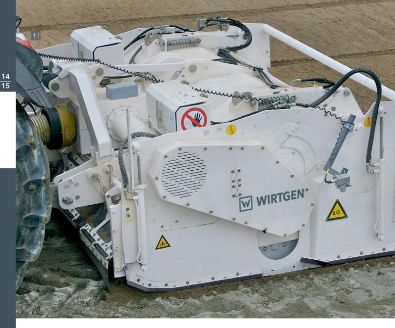
1 The milling and mixing rotor is the only part penetrating the soil. The current milling depth can be monitored on a digital milling depth indicator.
