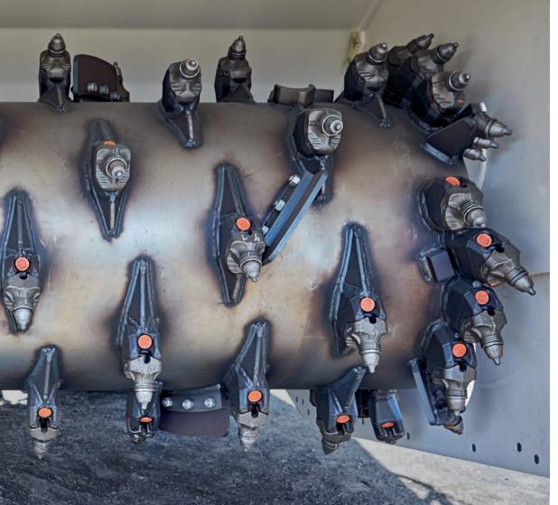
2 The quickchange toolholder system HT22 significantly reduces operating costs of the machine.
