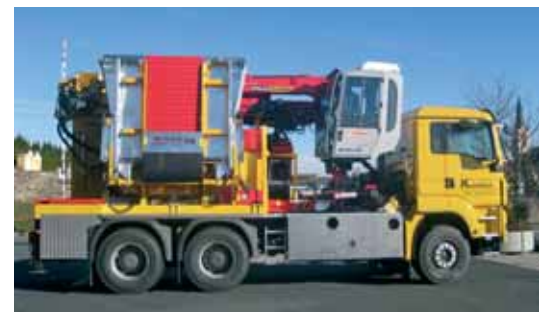
Timber crane with lifting crane cab
