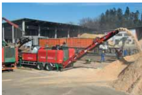
WT 10 DLB Longitudinal machine conveyor discharge (conveyor discharge)
