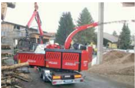
WT 10 on carriage with diesel engine John Deere 600 HP, chopping machine with slewing ring
