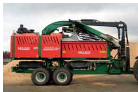
WT 10 DLK. WT 10 on carriage with diesel engine CAT C18 700 HP, chopping machine with slewing ring
