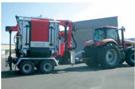
WT 11 Z with blower and ejector for tractors from 350 HP onwards
