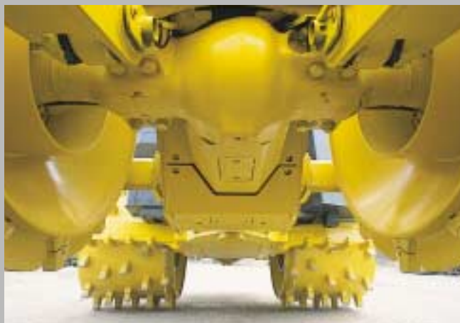
Protected axles, body guard and sealed wheels ensure highest durability.
