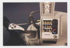
**Pilot Actuated Loader Joystick**
