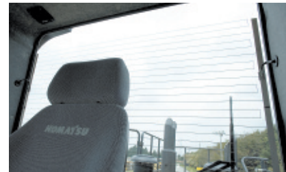
Rear heated glass provides clear view even in freezing or condensation conditions.
