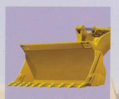
**High-Tensile Strength Steel Construction** -provides high wear resistance and excellent resistance to twisting and distortion when under heavy loads.
