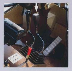
**Kickdown Switch -** Located on top of the boom control lever.
