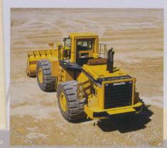
Electronic Display and Monitoring System-in the operator's compartment allows the operator to make prestarting checks from his seat.
