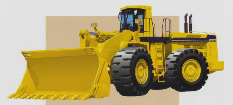
Flywheel Horsepower @ 2000 RPM 789 HP Operating Weight 204,124 lb Bucket Capacities 13.7 yd<sup>3</sup>
