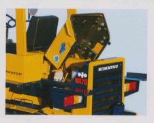
The full-tilt engine hood opens widely with a single touch, exposing the engine and hydraulic and other equipment for easy maintenance. The engine coolant level can be instantly checked by the radiator subtank.
