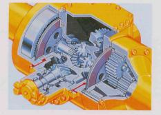
Sealed, wet, disc brakes are adjustment-free and protected from water, dust and other foreign elements. This results in sure braking performance at all times.
