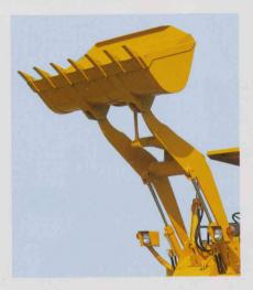
Z-bar loader linkage design assures dynamic digging force. This plus powerful traction enable the WA70-1 to excavate and scoop materials with speed and assurance. In addition, large dumping clearance and reach facilitate loading operations.
