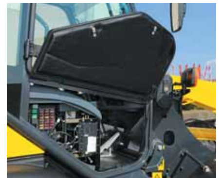
Side cover for quick maintenance access
