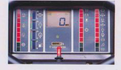
The electronic display and monitoring system: All important checkpoints are monitored and the operator is alerted through the sophisticated display panel in the event of a malfunction or emergency. The Electric System for Safety promotes foolproof operation.
