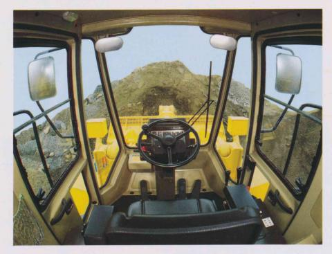
Spacious, comfortable cab (optional): The use of a cab with expansive tinted glass relaxes the operator and improves his visibility. Ergonomically arranged instruments, control levers and pedals boost operating efficiency. The cab is mounted on the rear frame with rubber pads to minimize noise and vibration.
