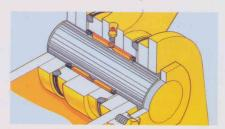
Sealed loader linkage pins and oil-lubricated pins need less maintenance. Bucket hinge pins are sealed-oil lubrication for extended refilling intervals of 2000 hours. Bucket linkage pins are lubricated and protected by dust seals and cord rings as are all loader linkage pins. As a result, lubrication intervals are greatly extended.
