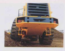
High machine stability: A center-pin-supported rear axle and large oscillation angle maintain level operation on even the roughest surfaces. This, plus a long tread and large static tipping load, give the WA600-1 high stability for efficient digging/carrying operations.
