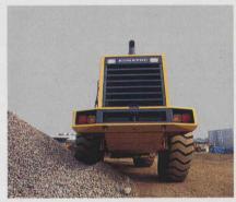
Demand valve steering system — guarantees smooth, constant steering regardless of engine speed. This not only provides easy machine operation, but also decreases the chance of load spillage.
