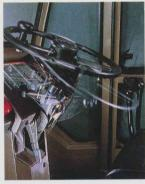
Tiltable steering column and adjustable oil suspension seat — The tiltable steering column can be adjusted along a wide range. Combined with the fully-adjustable oil suspension seat it allows the operator to obtain maximum comfort and efficiency during operation.
