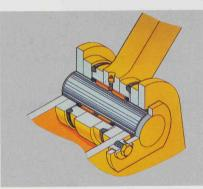
Sealed loader linkage pins — keep the grease in and contaminants out providing extended grease intervals. Also, the greasing points are conveniently located so that they are within easy reach.
