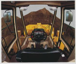
Spacious, comfortable operator's compartment — is rear-mounted to reduce operator swing and fatigue. The optional cab provides excellent visibility with a large area of tinted glass, and is rubberpad mounted to minimize noise and vibration. All pedals, control levers and instruments are arranged for maximum operating efficiency.
