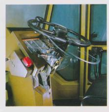
The steering wheel smoothly tilts within a 100 mm (4") range, offering ideal steering conditions for every operator.
