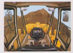
Spacious, comfortable cab (optional): The use of a cab with expansive tinted glass relaxes the operator and improves his visibility. Ergonomically arranged instruments, control levers and pedals boost operating efficiency. The cab is mounted on the rear frame with rubber pads to minimize noise and vibration.
