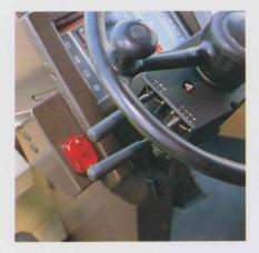
**Fingertip control** is realized with the electrically controlled transmission, assuring responsive, light-touch manipulation of the speed control and direction change levers provided on the side of the steering column.
