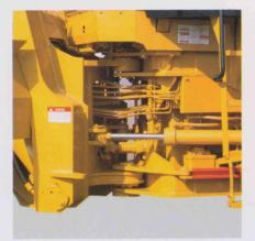
Smooth, light-touch steering and work equipment control: The demand valve system guarantees light-touch steering at all times. Pilot Operated Control (POC) through a pilot operated control valve assures lighttouch work equipment control and excellent fine control.
