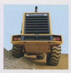
High machine stability: A centerpin-supported rear axle and large oscillation angle maintain level operation on even the roughest surfaces. This, plus a long wheelbase, wide tread and large static tipping load, give the WA500-1 high stability for efficient digging/carrying operations.
