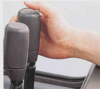
Servo-assisted two-lever hydraulic control, with "kickdown".
