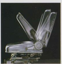
Oil-suspension seat (optional): The seat is up/down and fore/aft adjustable with cushion hardness also varying according to the operator.
