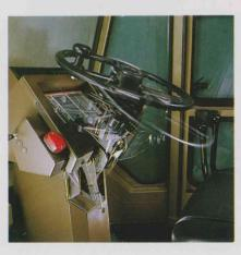
The steering wheel smoothly tilts within a 100 mm (4") range, offering ideal steering conditions for every operator.
