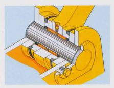
Sealed loader linkage pins need less maintenance. Bucket hinge and linkage pins are lubricated and protected by dust seals and cord rings as are all loader linkage pins. As a result, lubrication intervals are greatly extended.
