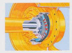
Wet, multiple-disc brakes are adjustment-free. Sure braking performance is maintained even when the machine is operated on muddy terrain. The torque proportioning differential minimizes tire slippage for extended tire life.
