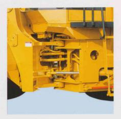
Smooth, light-touch steering and work equipment control: The demand valve system guarantees light-touch steering at all times. Pilot Operated Control (POC) through a pressure proportional control valve assures light-touch work equipment control and excellent fine control.
