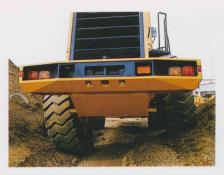
High machine stability: A centerpin-supported rear axle and large oscillation angle maintain level operation on even the roughest surfaces. This, plus a long wheelbase, wide tread and large static tipping load, give the WA450-1 high stability for efficient digging/ carrying operations.
