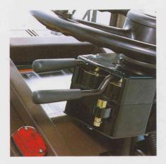
**Fingertip control** is realized with the electrically controlled transmission (ELECTRAN), assuring responsive, light-touch manipulation of the speed control and direction change levers provided on the side of the steering column.
