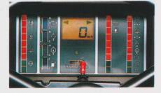
The electronic display and monitoring system (EDIMOS): All important checkpoints are monitored and the operator is alerted through the sophisticated display panel in the event of a malfunction or emergency. The Electric System for Safety (ESS) promotes foolproof operation.
