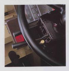
Fingertip control is realized with the electrically controlled transmission, assuring responsive, light-touch manipulation of the speed control and direction change levers provided on the side of the steering column.
