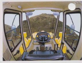
Spacious, comfortable cab (optional): The use a cab with expansive tinted glass relaxes the operator and improves his visibility. Ergonomically arranged instruments, control levers and pedals boost operating efficiency. The cab is mounted on the rear frame with rubber pads to minimize noise and vibration.
