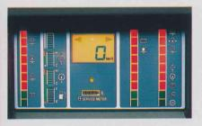
The electronic display and monitoring system: All important checkpoints are monitored and the operator is alerted through the sophisticated display panel in the event of a malfunction or emergency. The Electric System for Safety promotes foolproof operation.
