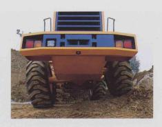
High machine stability: A centerpin-supported rear axle and large oscillation angle maintain level operation on even the roughest surfaces. This, plus a long wheelbase, wide tread and large static tipping load, give the WA350-1 high stability for efficient digging/ carrying operations.
