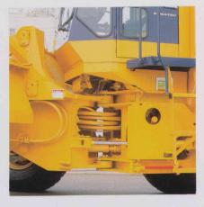
Smooth, light-touch steering: The demand valve system guarantees light-touch steering at all times. An advanced hydraulic design in the steering circuit gives the WA350-1 a smooth steering action and maximizes operator comfort while minimizing soil spillage.
