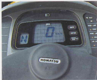
The main monitor keeps the operator constantly informed on the various travelling functions.
