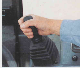
The servo-controlled single-lever hydraulic system with kick-down system.
