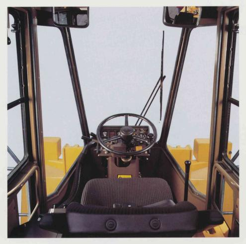
**Superior Visibility** – 47% of the total cab area is tinted glass, giving the operator a clear and complete view of the working environment. This greatly increases the operator's confidence and productivity.
