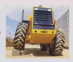
High machine stability: A centerpin-supported rear axle and large oscillation angle maintain level operation on even the roughest surfaces. This, plus a long wheelbase, wide tread give the WA150-1 high stability for efficient digging/carrying operations.
