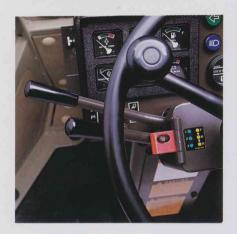
The speed control and direction change levers provided on the side of the steering column assure responsive, light-touch manipulation.
