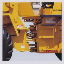
Smooth, light-touch steering: The priority valve system guarantees light-touch steering at all times. An advanced hydraulic design in the steering circuit gives the WA150-1 a smooth steering action and maximized operator comfort while minimizing soil spillage.
