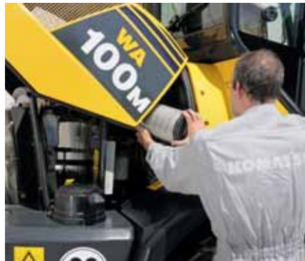
Convenient air filter access
