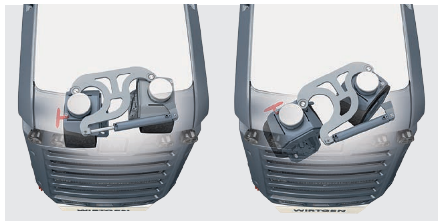
Detailed view of the four-wheel front axle.
