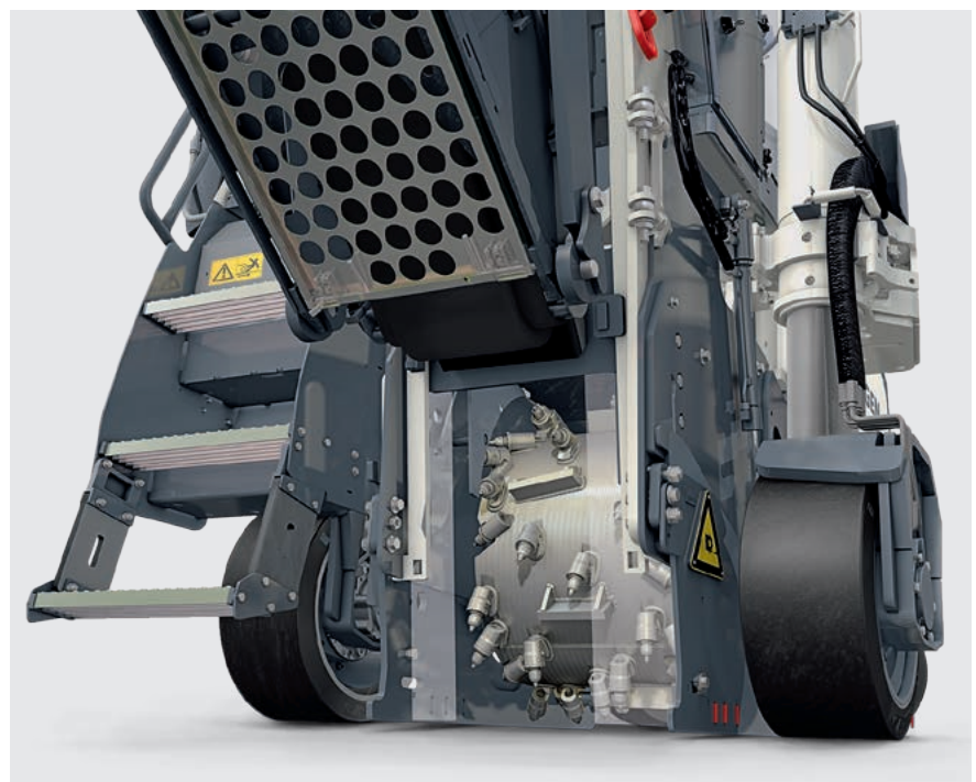
Milling drum unit with intelligent features.
