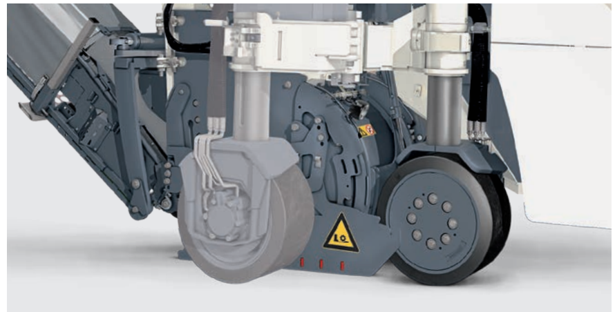
Quick pivoting of the right-hand rear wheel.
