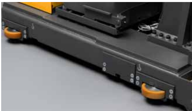
Complete package for rail- or wireguided steering.
