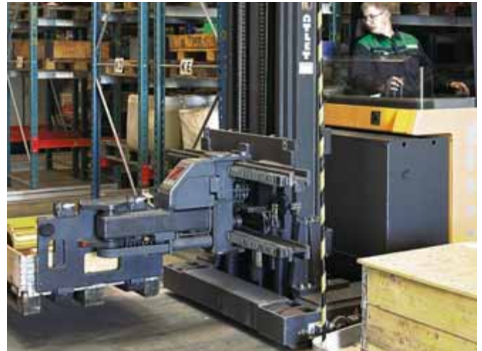
Autostop for safety. Stops the truck automatically at the ends of the aisle.
