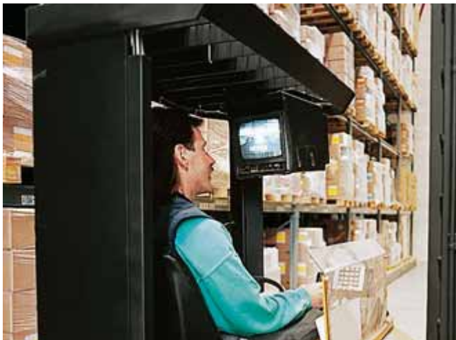
Video equipment. One or more cameras, gives a clear view of the position of the pallet.
