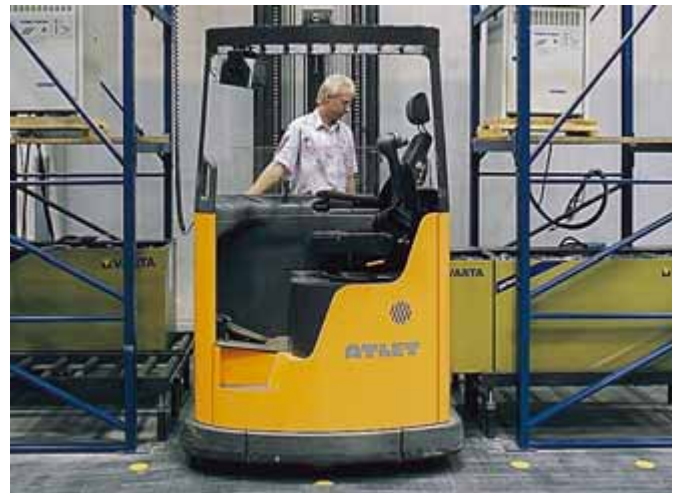
Powered battery change for multi shift operation.
