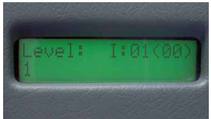
Automatic level selector. The driver enters the shelf level via the keyboard and the truck raises the load to the correct level. Light indicator to show the exact position of the truck in the aisle.
