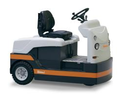
3-wheel tow tractor, man on board, with rear-wheel drive. Extremely compact and easy to drive, ideal for all industrial duties -both indoors and outdoors.
