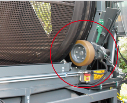
Fast replacement of drums and conveyor belts: Roller drive of screen and conveyor belts in „Quick replacement cartridges“
