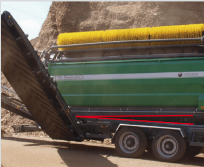
Hydraulic inclination adjustment of screen for optimizing the throughput rate and material classification
