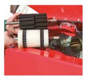
Easy change-around between coarse and fine metering wheels
