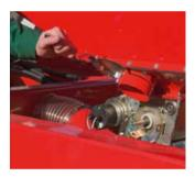
Exit shutter to empty seed tank completely
