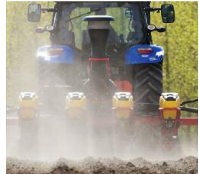
Elevated air intake greatly reduces the risk of dust problems. Available as an option.
