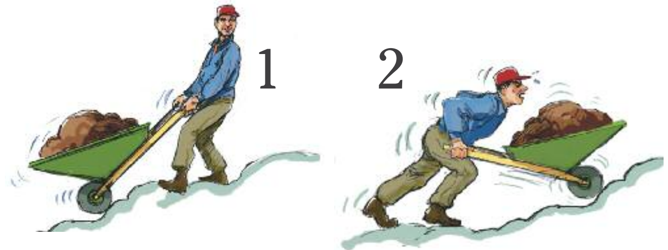
The carrying wheels on Tempo are trailed (1) instead of pushed (2), which is the usual solution on precision seed drills. The great advantage with trailed carrying wheels is that the machine is easier to draw and that the vibrations in the row units decrease.
