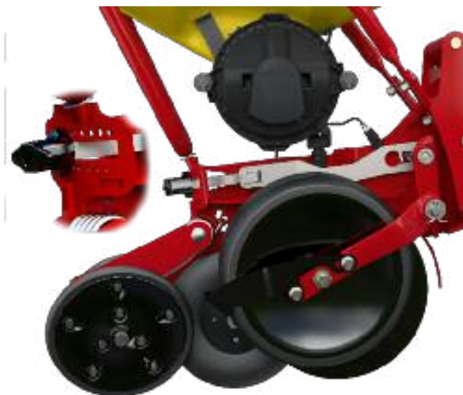
Drilling depth is easy to set with a lever that controls the relationship between carrying wheel and seed. The great advantage with trailed carrying wheels is that the machine is easier to draw and that the vibrations in the row units decrease.
