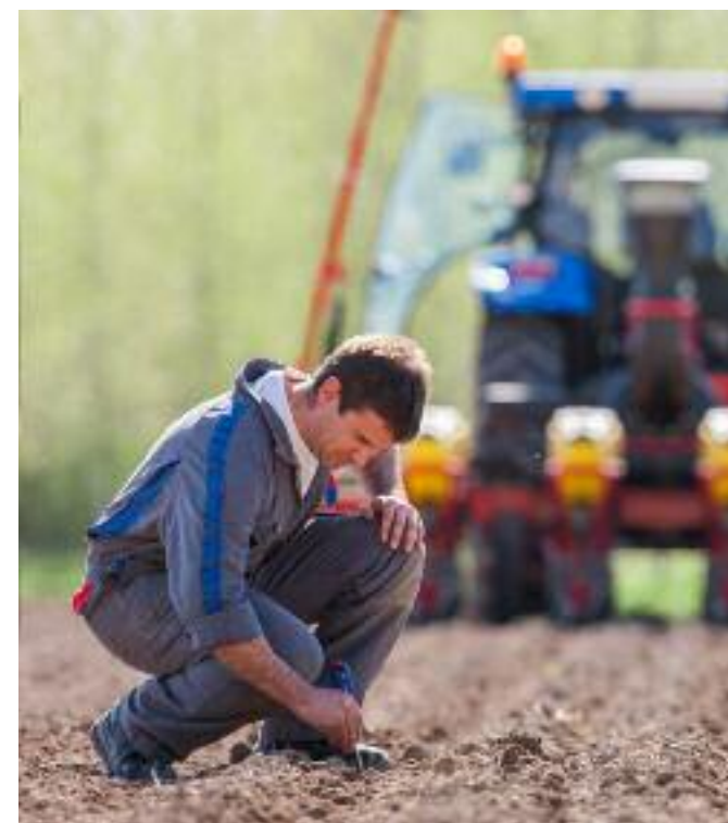
Drilling depth is easy to set with a lever that controls the relationship between carrying wheel and seed. The great advantage with trailed carrying wheels is that the machine is easier to draw and that the vibrations in the row units decrease.
