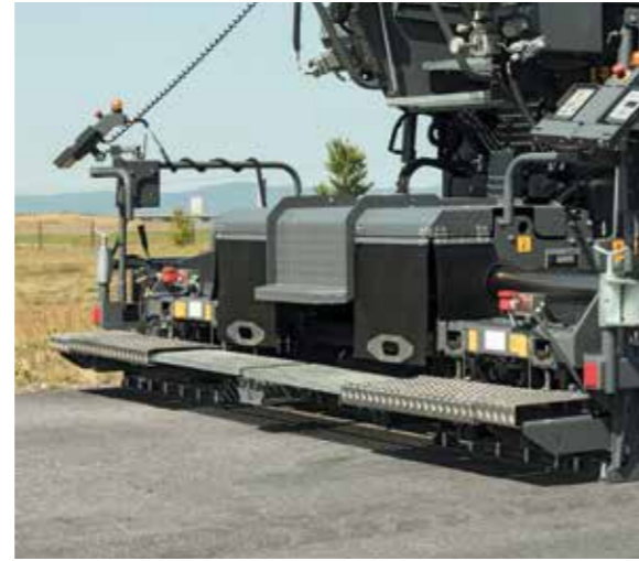
AB 340 Extending Screed with 25cm bolt-on extensions
