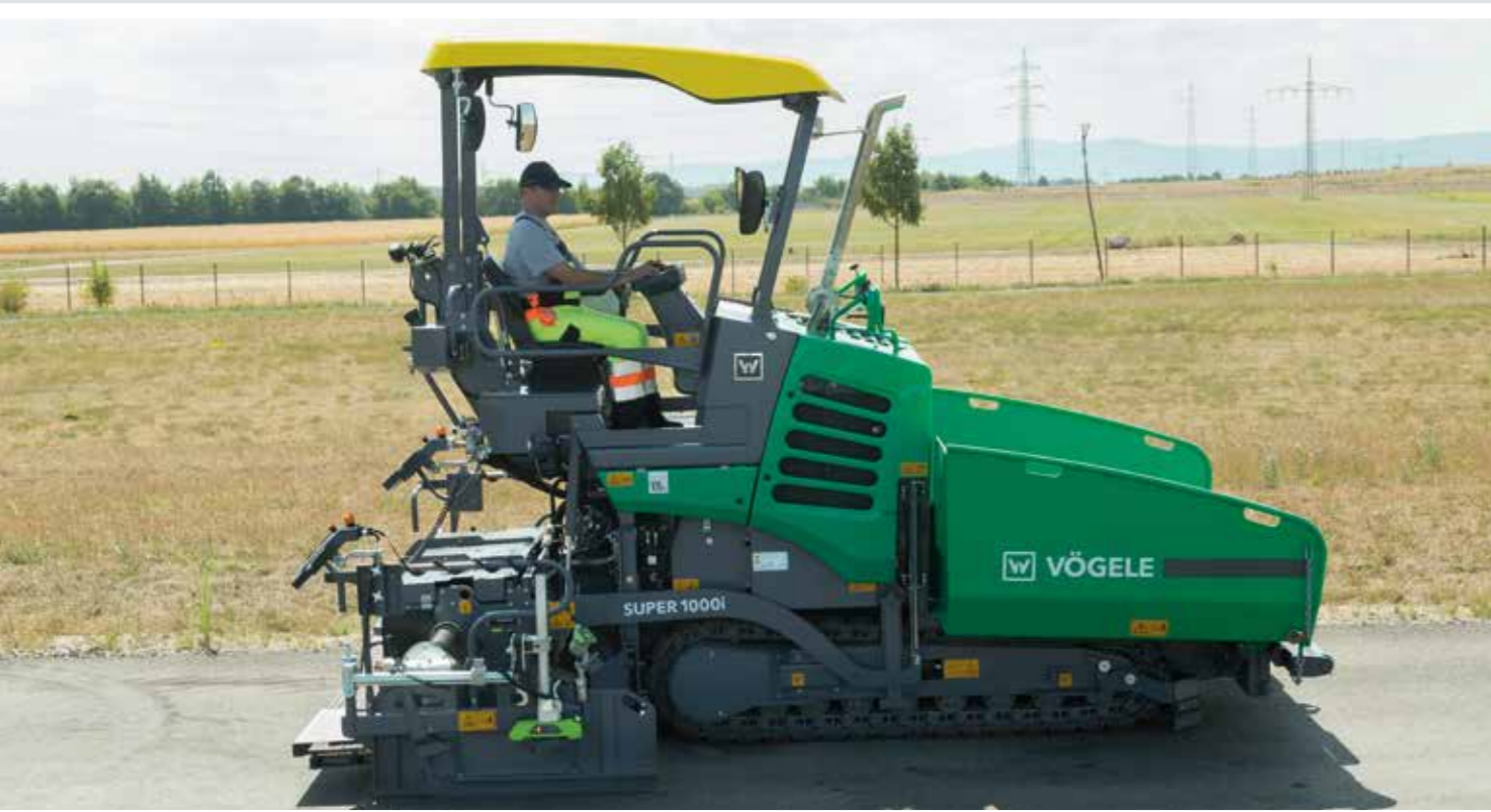
The power unit of the SUPER 1000i with diesel oxidation catalyst (DOC) for exhaust gas after-treatment complies with the strict requirements of European exhaust emissions standard Stage 4 and US EPA Tier 4f.
