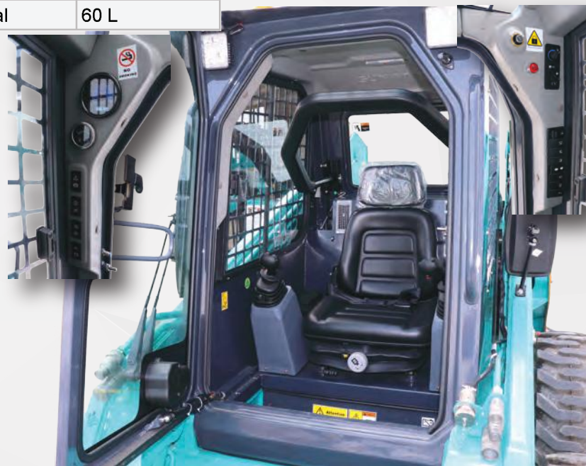
Enclosed cab offers air conditioning and LCD Touchscreen for optimal working
