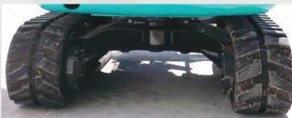
Telescopic Chassis gives the operator the ability to navigate tight spaces easily
