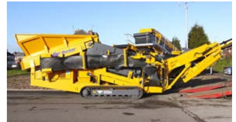
Conveyors folded ready for transport.
