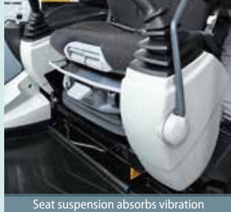
Seat suspension absorbs vibration
