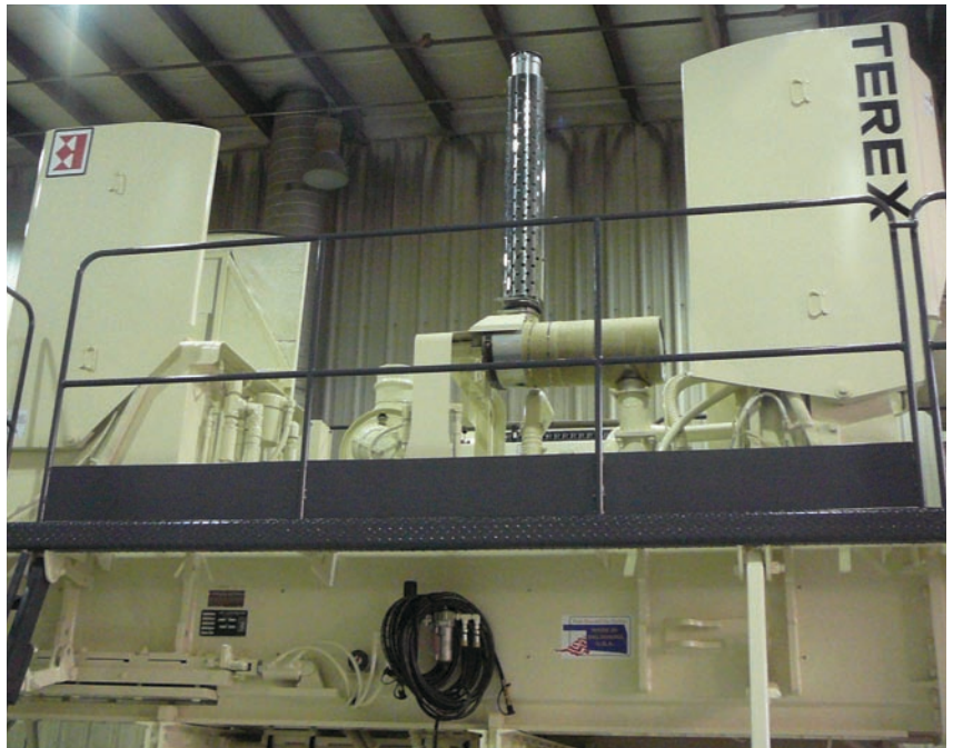
Powered flip-up cowling allows full access to engine compartment.
