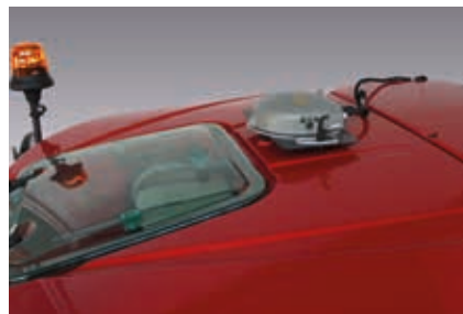
The satellite antenna placed on the cab roof receives the GPS signal.
