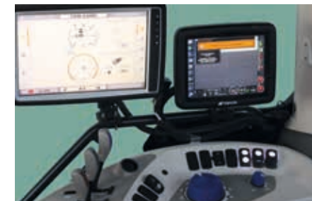
The 8.4" touch screen monitor for management of satellite-based guidance and ISOBUS system.
