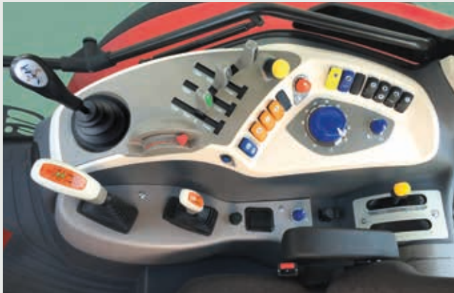
Cab interior on version with Xtrashift transmission: tractor controls are placed on the right-hand side console.
