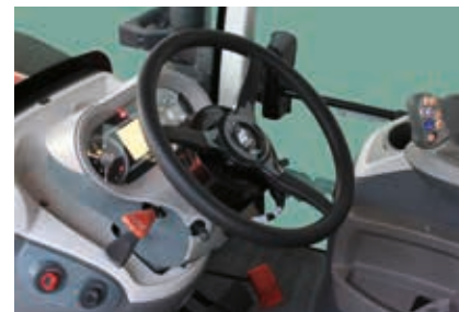
The electronic steering wheel allows precise steering delivering up to 2cm pass-to-pass accuracy.
