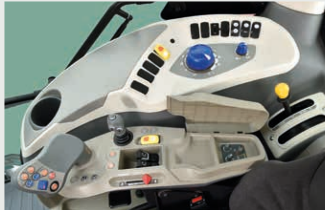
Cab interior on version with VT-Drive transmission: tractor controls are placed on the right armrest of the driver's seat.
