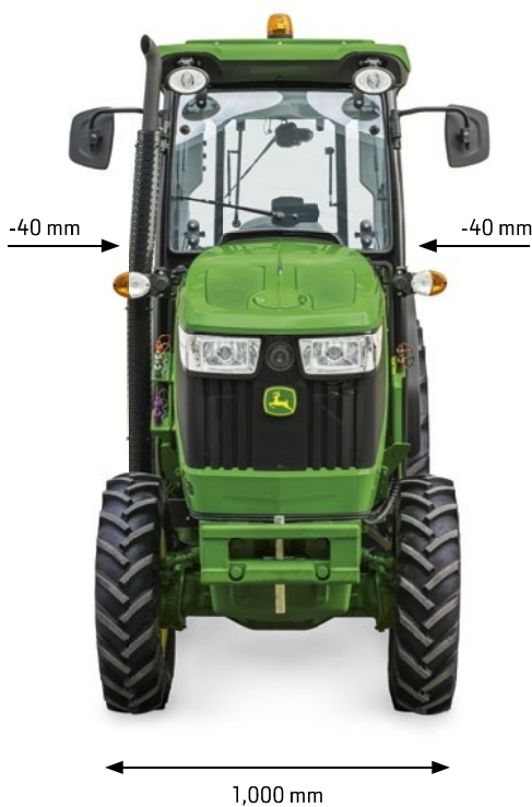
on 5GN, 5GF and 5GV No more than 1 m in overall width, this new cab avoids damaging foliage and grapes in super-narrow vineyard rows.
