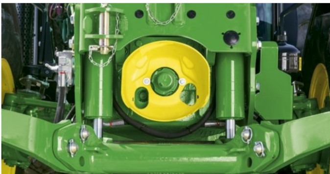
Optimized PTO Runs at 1,000 rpm to power even heavy implements.
