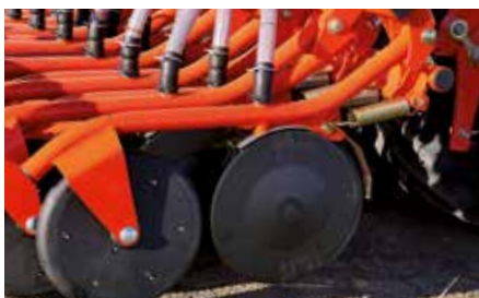
The Kubota CD-coulters consist of two steel discs (Ø410mm) with 12.5cm row spacing. Perfect depth control is ensured by the press wheels (Ø 380mm).
