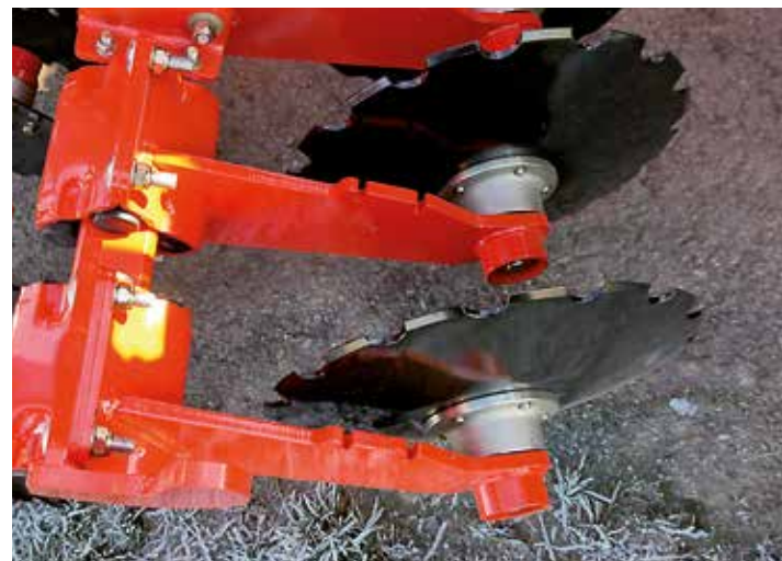
The first disc row ensures good penetration and prevents blockages. The second row works offset and takes over the soil flow and plant residues of the first row.
