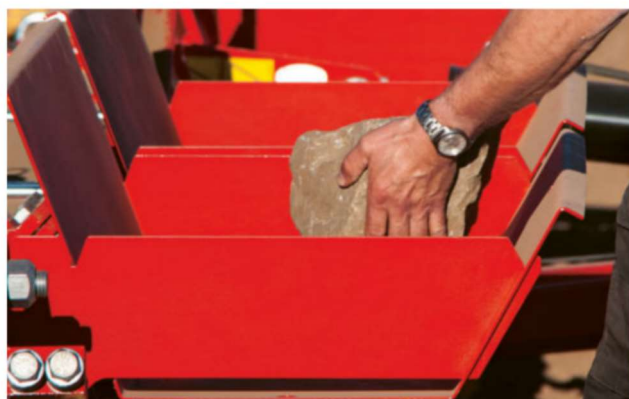
The stone trays fitted on Rollex, stones can be picked up directly from the field.
