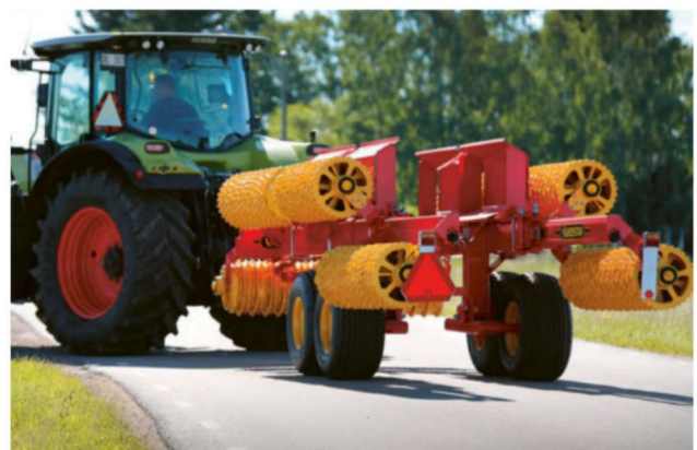
The folding technique of the roller lowers the centre of gravity, making transport safer. Despite Rexius' wide working width, the transport width is 2.5 metres.
