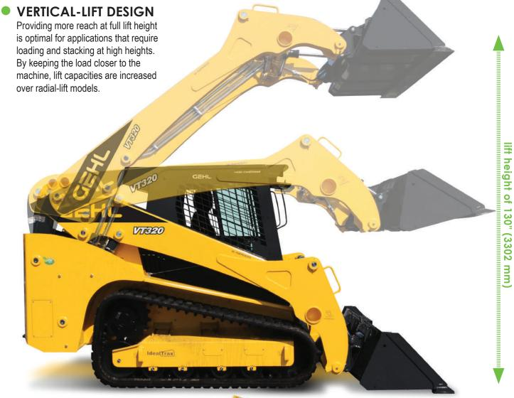
**TRUE VERTICAL** The VT320 has a true vertical lift path of almost 11 feet.
