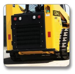
**COUNTERWEIGHT/BUMPER** Gain extra tipping capacity while offering increased rear protection. Increases rated operating capacity on RT165 by 100 lbs. (46 kg) and adds 1.5" (38 mm) to overall length.
