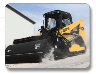
ADAPTED SKID LOADER CHASSIS Custom built from the proven design of the R165 skid loader to aid in superior weight distribution. This design enhances stability, grading, tractive effort, and ride control.
