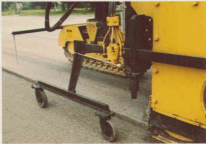
HYDRA-MATION Grade & Slope Control provides superior profiling accuracy.
