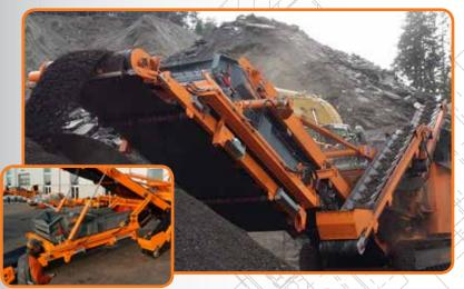
Hydraulic cylinders on the screenbox save maintenance time.
