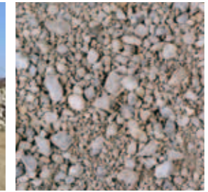
Recycled concrete aggregate
