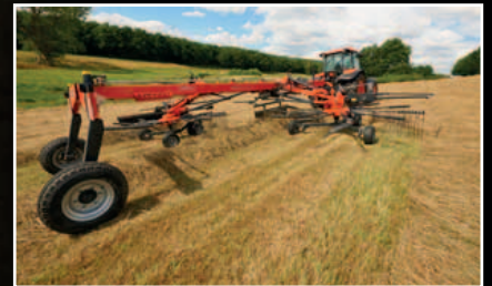
Pivoting pulled front wheels protect the rotor from going into the ground.
