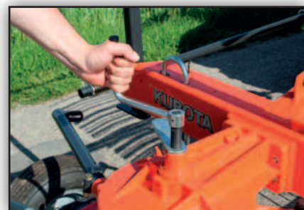
Easy setting of correct rotor height.
