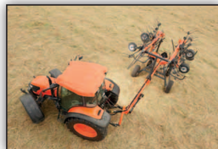
80° turning angle ensures excellent manoeuvrability.
