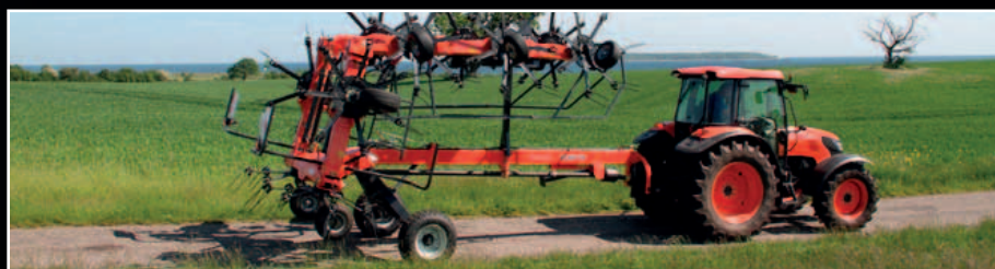
During transport both tedders have a height of 11'2" (3.4m) and a width below 9'10" (3.0m).
