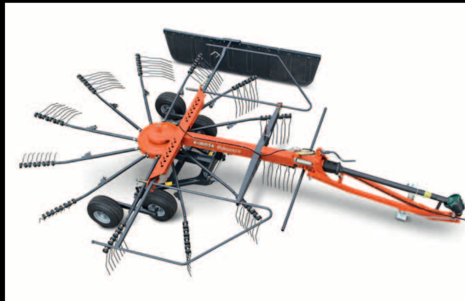
RA1047T - trailed, low input rake, yet still delivering 15'1" (4.6m) working width.
