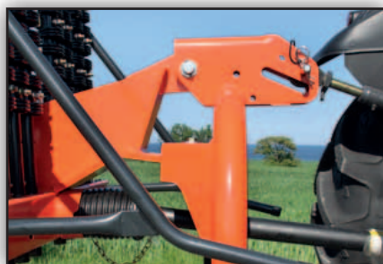
A pivoting 3-pt headstock ensures perfect ground following.
