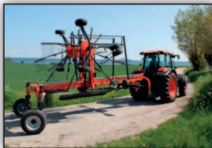
To limit transport height further, the tine arms can be removed. The swath board folds up automatically.
