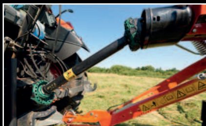
Wide angle PTO shaft - for increased maneuverability.
