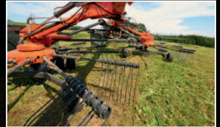
Generous overlap between rotors ensure clean raking.
