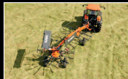
SideShift to the left - raking without driving on unraked crop.
