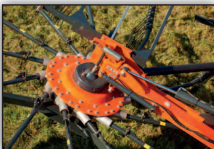
Hydraulically adjustable working width between 24'11" (7.6m) and 27'7" (8.4m).
