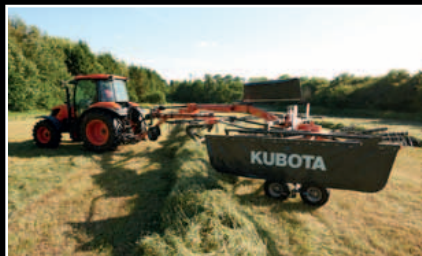
With 20" (50cm) lifting height, swaths are easily crossed.
