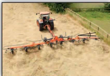
For border tedding the outer rotors are pivoted, to secure evenly inward spreading.
