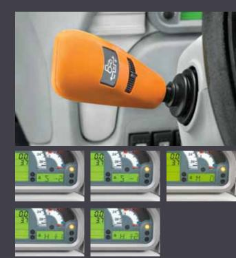
comfort and convenience, gear changes can also be made smoothly and effortlessly using the "Comfort Clutch" button on the knob of the shift lever, without having to depress the clutch pedal.
