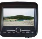
The advanced new cluster with 7 inch wide color LCD screen and toggle switch allows the operator to select his personal machine preferences. Power and work mode selection, self diagnostics, optional rear-view camera, maintenance check lists, start-up machine security, and video functions were integrated into the cluster to make the machine more versatile and the operator more productive.
